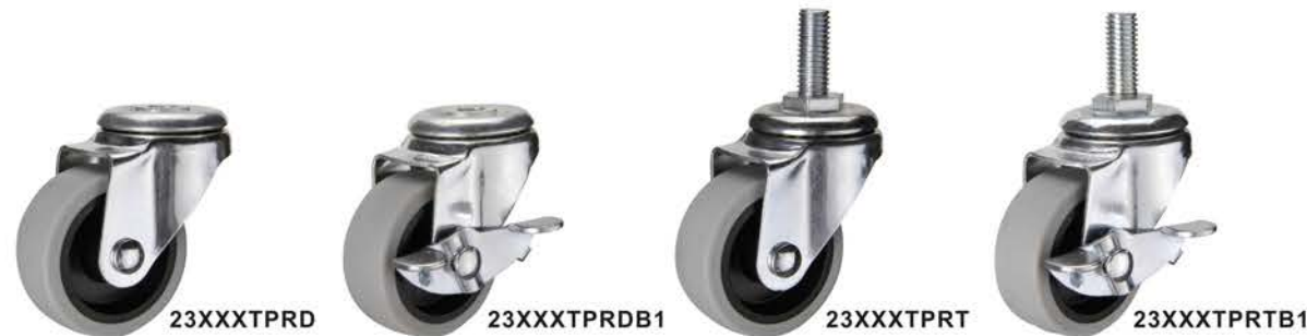
TPR wheel , Plain bearing, Hardness : 85 ± 5 Shore A ,Temperature range: - 5°C~80°C
