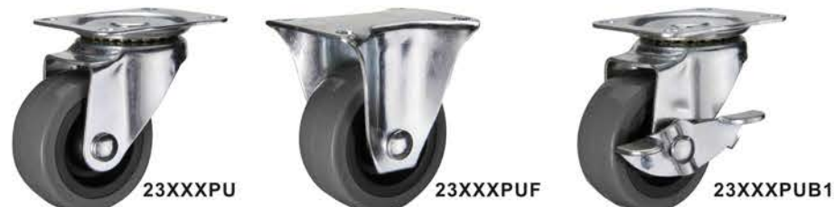
Polyurethane wheel , Plain bearing , Hardness :90 ± 5 Shore A , Temperature range : -5°C~80°C
